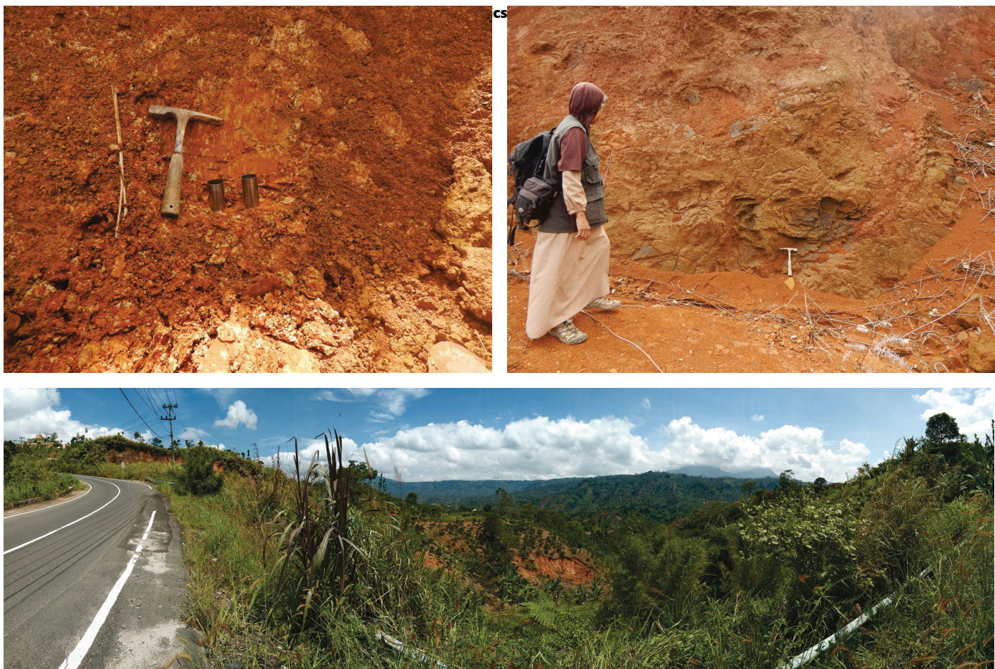
Fig. 4. Tropical volcanic residual soil. A. Reddish-brown color and loose characteristics at S5 location. B. Hard surface characteristic at X33 location. C. Groove erosion at S10 location
